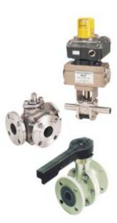
An extensive range of full and reduced bore ball valves serving a wide spectrum of applications in the chemical, pharmaceutical, oil, petrochemical and allied process industries. Available as lined, flanged, wafer and screwed/welded, metal or soft seated incorporating either floating or trunnion mounted designs for shut-off or control. Also suitable for cryogenic and corrosive services.
